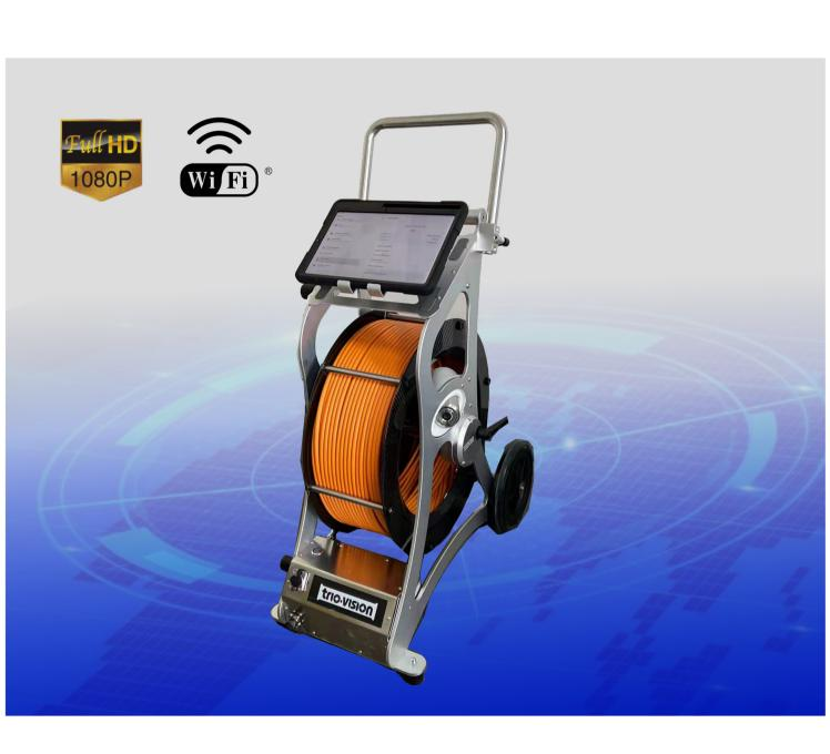
TVS-50 Pushrod Camera Inspection System is a special tool for inspecting pipeline located in municipal or commercial or residential areas, with the diameter ranging from DN50 and typically upto DN150. As a portable tool, the system has high-definition video and is connected by WiFi for long distance operation.
